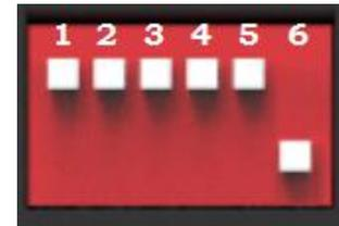
**The address is configured follow ASCII code: ("X" is terminal resistance).**
