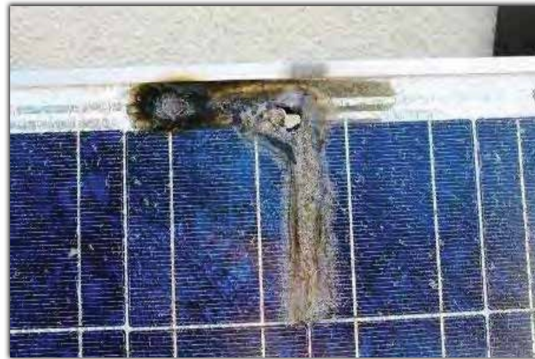
Hot-Spots Damage cells and panels
