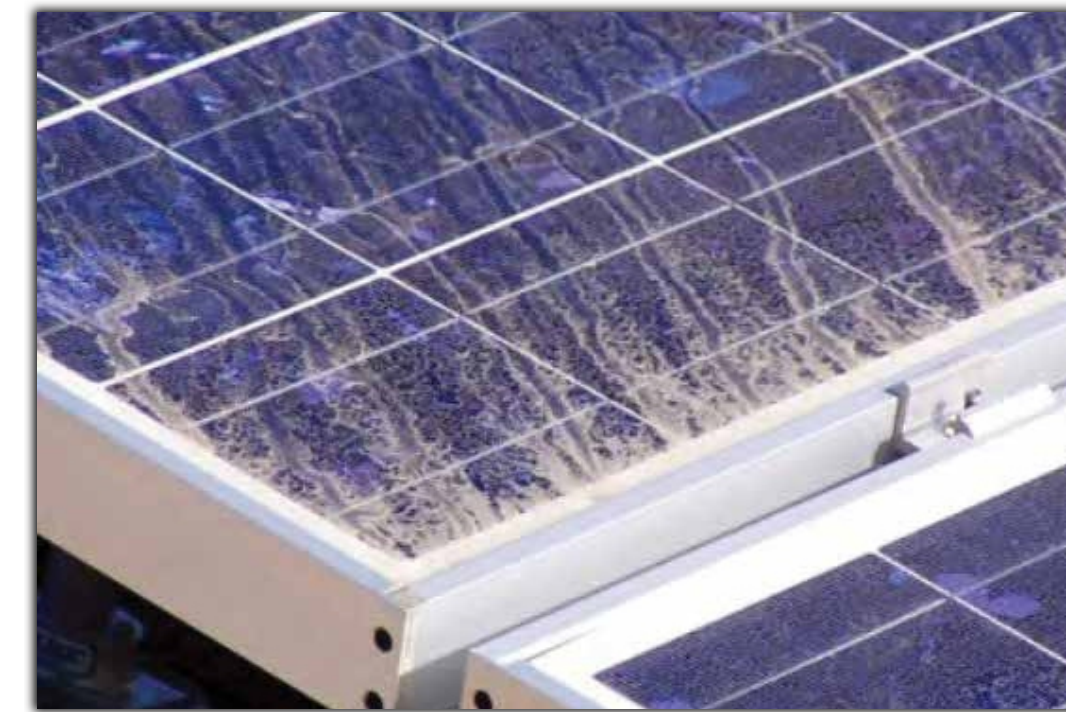
Dirt, dust and shading lead to Hot-Spots
